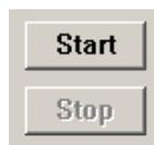
When the Start-button is pressed a Slow Kinetics recording is started by an  $F_o$ ,  $F_m$ -determination. It can be terminated at any time by pressing the Stop-button.
