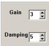
The **Gain** relates to the amplification of the fluorescence signal. It can be changed between 9 settings, with the standard setting 3. Please note that the signal/noise ratio is not changed by the Gain setting. For optimal results it is recommended to choose a high setting of Measuring Light intensity (e.g. standard setting 9) and then adjust the signal amplitude to ca. 400 units.
