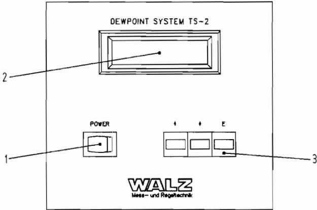
Fig. 2: Frontplate of the Control and Display Unit TS-2
