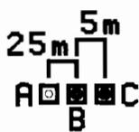
**Jumper position 5 m** (jumper between B and C) for cables of length < 10 m, e.g. for cable TS-K5
