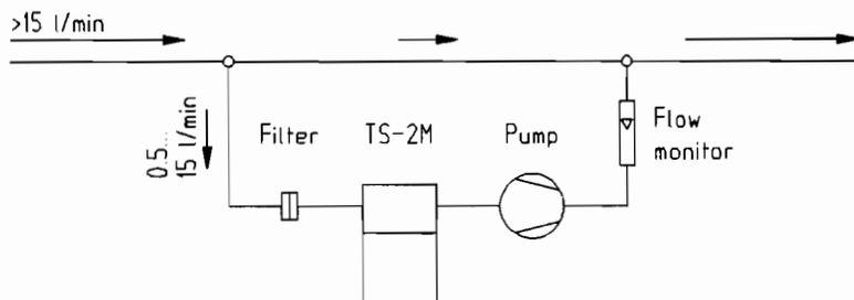
Fig. 5: Integration of the Dewpoint Mirror Measuring Head TS-2M in a pneumatic system with a measuring gas flow greater than 15 l/min
